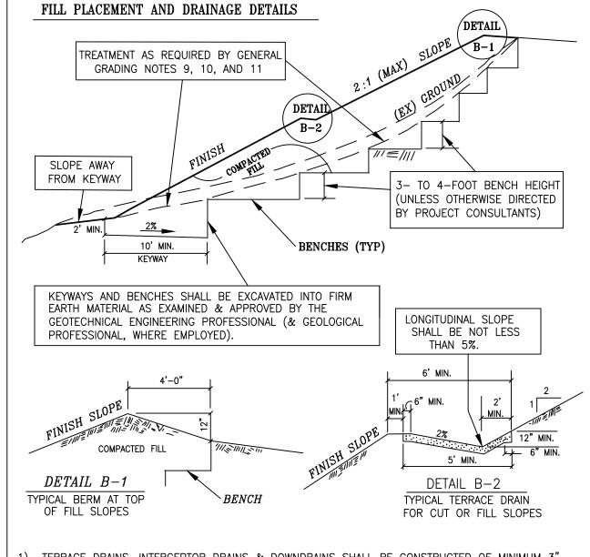
1) TERRACE DRAINS, INTERCEPTOR DRAINS & DOWNDRAINS SHALL BE CONSTRUCTED OF MINIMUM 3" CONCRETE OR GUNITE REINFORCED WITH 6x6—W1.4XW1.4 WELDED WIRE FABRIC.
