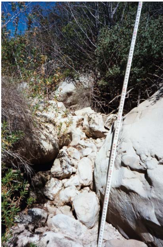
Side channel around barrier #65 in Old Man Creek. Visible portion of stadia rod is approximately 9 ft long. See Figure 3 for location and Table 2 for barrier details.
