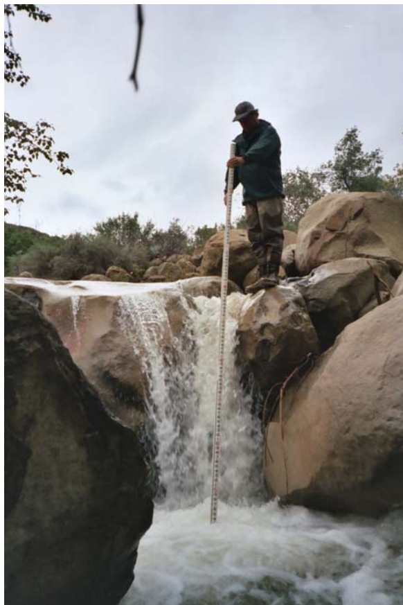
Barrier #625 in Murietta Creek, April survey. Visible portion of stadia rod is approximately 10 ft long. See Figure 3 for location and Table 2 for barrier details.
