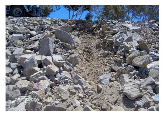
Photo 5: Test pit SCR-1-TP3. Looking perpendicular to levee. Note coarser revetment.
