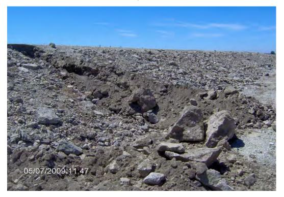
Photo 4: Test pit SCR-1-TP2. Looking downstream. Note fine material in trench and larger material at toe.
