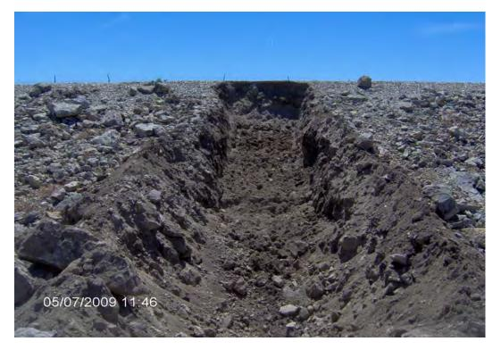
Photo 3: Test pit SCR-1-TP2. Looking perpendicular to levee. Note fine material.
