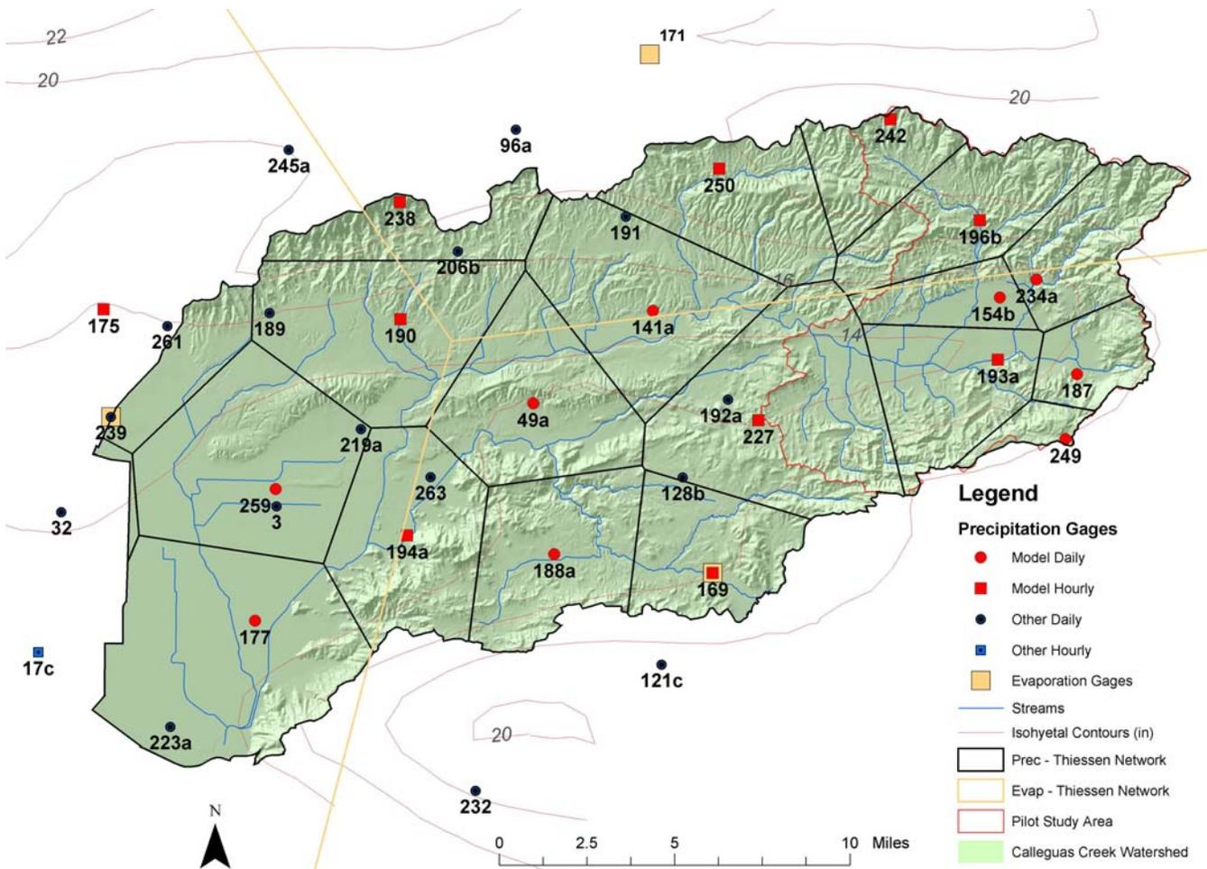
Figure 2.1 Ventura County Precipitation Gages in or near the Calleguas Creek Watershed
